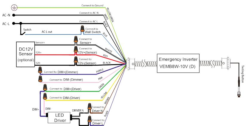
3. For luminaire with non-dimming LED driver (\* LED DRIVER INPUT POWER NOT GREATER THAN 8W)
