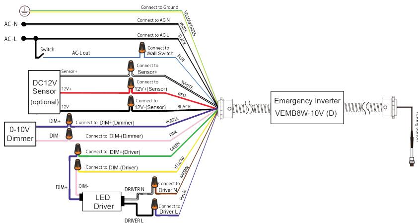
2. For luminaire with 0-10V LED driver, without using 0-10V dimmer (\* LED DRIVER INPUT POWER NOT GREATER THAN 60W)
